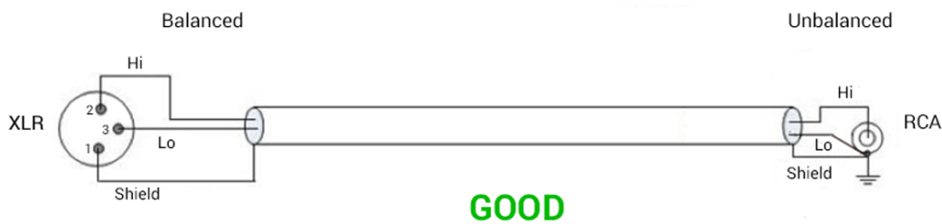
Figure 2 Correct balanced output to unbalanced input connection method
