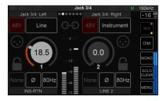
You are now ready to record your External insert return channel. It is common practice to record the direct Mic PreAmps channel #1 along with the Processed Hardware Insert #3 return.
