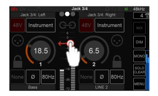
The Preamps controls for those inputs 3-4 are similar to inputs 1-2 but will apply to Hi-Z, Instruments or Line inputs types only. Thus, the 48V Phantom power and Pad/Boost options are not available for the Anubis inputs 3-4.
