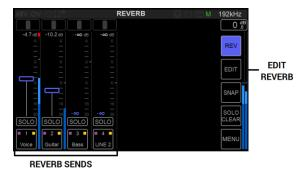
Tap the EDIT button to open the REVERB UI in order to adjust the Reverb parameters
