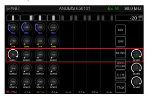
Note: Sends 1 to 3 include a Master Send level at the fast right of the Remote Web Access Mixer.
