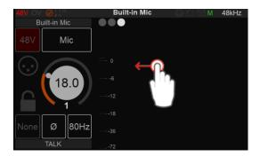
The Preamps controls for the Input 5 will control the built-in Talkback microphone.
