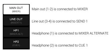
Warning: Routed output channels cannot be used twice. Once a routed channel is routed it cannot be used by another Mixer bus, re-using it would disconnect it from the Bus where it is in use.
