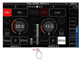
Swipe from left to the right in the PreAmps page to access the peered PreAmps. Note: Peered modules PreAmps might not support some parameters (Cut, Lock, Boost)
