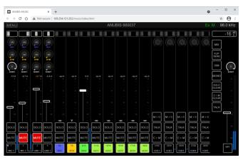
Web User Interface Page is a replica of the Anubis TFT display and allows the operator to remote control the Anubis from any web browser interface connected to the same network as Anubis
