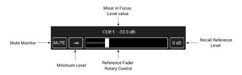
Refer to the Settings section in order to determine the reference listening level you wish to establish when recalled. By default, reference level is set to -20 dB and can be configured from the Anubis Settings>Monitoring where a value range of -144dB to +6dB can be selected.
