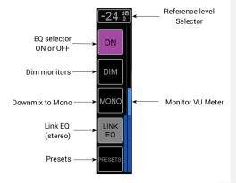
stereo linked channels, then enter the EQ with each channel and do not apply the Link EQ options.
