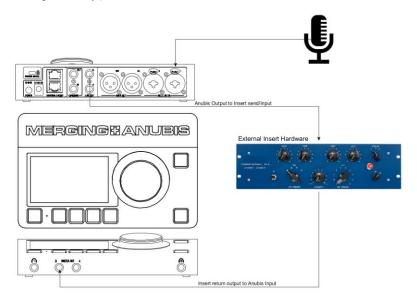
Find here below the procedure to accomplish external insert processing with the Music Mission. In the example here a microphone will be used as the source input. This one can as well go through an Insert to be recorded back with or without the Insert applied
