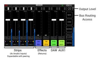
9. Open the Bus Routing Page and patch the Mixer and Mixer-ALT to the outputs you wish to monitor from.
