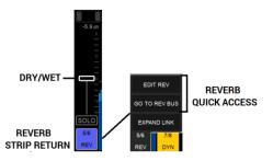
Note: You will need increase the Reverb return input level in order for the Reverb signal to enter back into your mixer. The fader will then act as a Dry/Wet global parameter.
