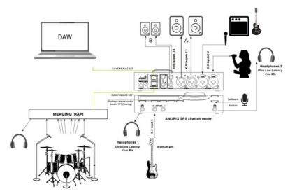
Setup example: Merging Hapi has been peered in Anubis, so that a Hapi AD Module (PreAmps Drum Mics) are mixed within the Anubis ultra-low latency engine, thus in the performers' Cues.
