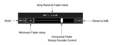
In order to reset the fader to the default 0dB value open the Horizontal Fader view by tapping the 0dB box on the fader section. This will also reset the Peak Hold that was present for that Strip channel inputs
