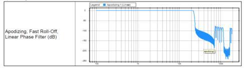
Brickwall: Ensures rejection of more than -100dB at Nyquist (0.50 x FS, 24 kHz @48k). Latency of 35 samples
