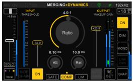
The Anubis Built-in Dynamics includes multi-modules. 1 X Gate, 1 X Compressor and 1 X Limiter that can be combined in series. With each module having its own parameter values. Limit your outputs buses or strip channel, apply compression to your strips, gate your snares or kick, compress and limit your vocals, compress your drums in parallel and more. The Dynamics can operate in Mono or Stereo mode (Link Dyn)
